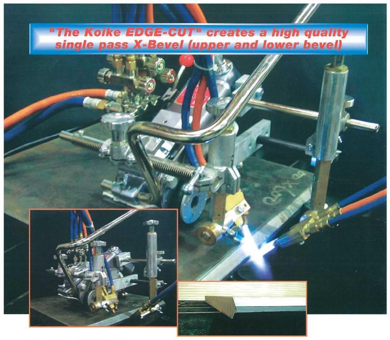
"The Koike EDGE-CUT" creates a high quality single pass X-Bevel (upper and lower bevel)
