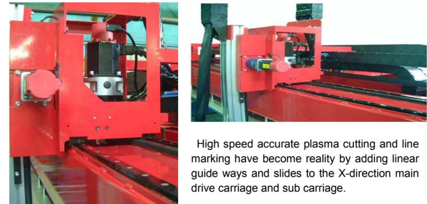
High speed accurate plasma cutting and line marking have become reality by adding linear guide ways and slides to the X-direction main drive carriage and sub carriage.
