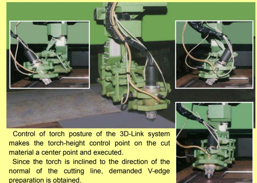
Control of torch posture of the 3D-Link system makes the torch-height control point on the cut material a center point and executed.
