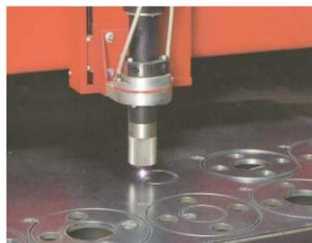
A vertical cutting within  $\pm 1.5$  degrees is obtained by using SUPER series. The upper edge of cut surface does not have roundness compared with any other plasma system. The longevity of the tip by which the insulation structure is assumed to be a feature is very long, and the longevity of the electrode is also long enough because of the gas control.
