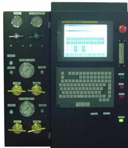
Centralized control station groups all control and operating functions in a single location, convenient to the operator.
