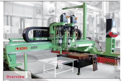
Replacing the Gas/Plasma Piercing by the Drilling, the piercing failures can be eliminated. The total processing time till the cutting completion can be shortened. I addition, thick plate piercing process by gas which requires skilled technology have been simplified, and it is also lead to increase the life time of nozzle and cutting tip.
