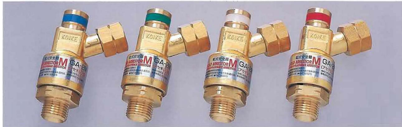
This MK series also has a dry thermal detection circuit breaker equipped with a thermal detection cutoff valve. In addition to the built-in non-flashback and non-return valve mechanism, it features a double safety function that detects an abnormal rise in temperature and interrupt the supply of gas, even in the event of a gas leak.
