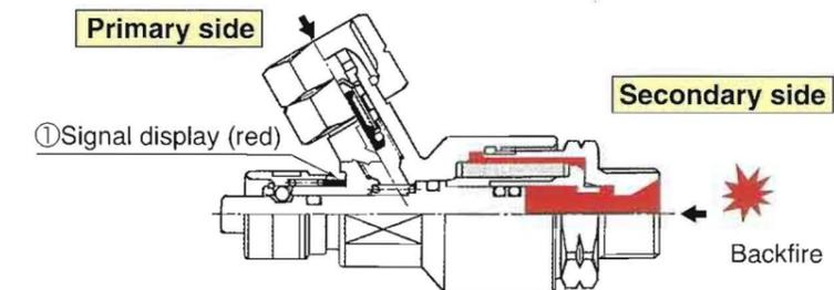
At the time of the backfire, the cutoff valve is pushed; then, the lock pin is pushed out and locked. To reset, press down the lock pin and then pull it back.
