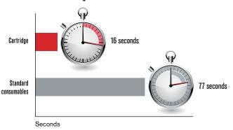
Based on a typical consumable changeover of electrode and nozzle.
